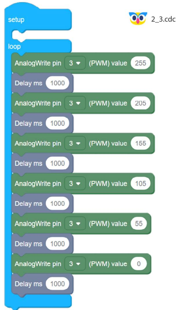
The image shows a Scratch code block for an Arduino project. It starts with a 'setup' block and a 'loop' block. The loop contains six pairs of 'AnalogWrite pin 3 (PWM) value' and 'Delay ms 1000' blocks. The PWM values decrease from 255 to 0 in increments of 50. A small owl icon and the text '2\_3.cdc' are visible in the top right corner of the code area.
